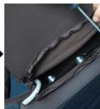
Make sure that the screws are inserted straight into the holes.
